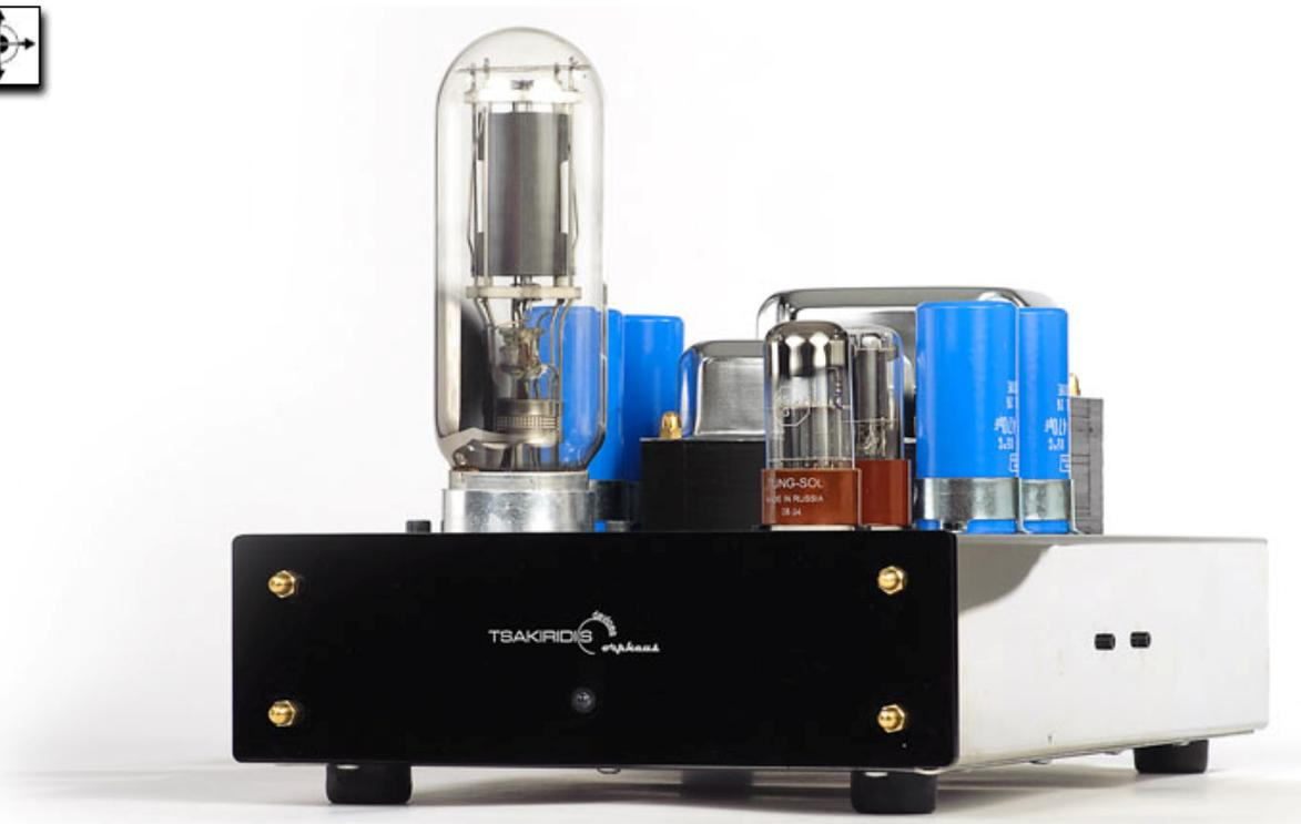
Rated at 25 watts, the class A zero feedback 845 Orpheus SET Orpheus runs three valves each, one 845 output valve, one 6SN7 and one 6SL7. The Tsakiridis product catalogue thankfully provided in English by Ikon Audio consultants lists further details such as gold-plated WBT i/o connectors, low-tolerance 1% metal film resistors, high-grade polypropylene signal capacitors, porcelain tube bases, United Chemicon power supply capacitors and hand-wired construction.
